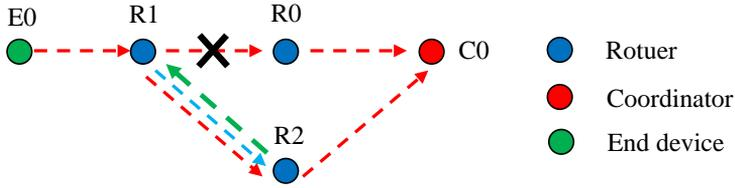
Fig. 4 Self-healing function of AODV algorithm
