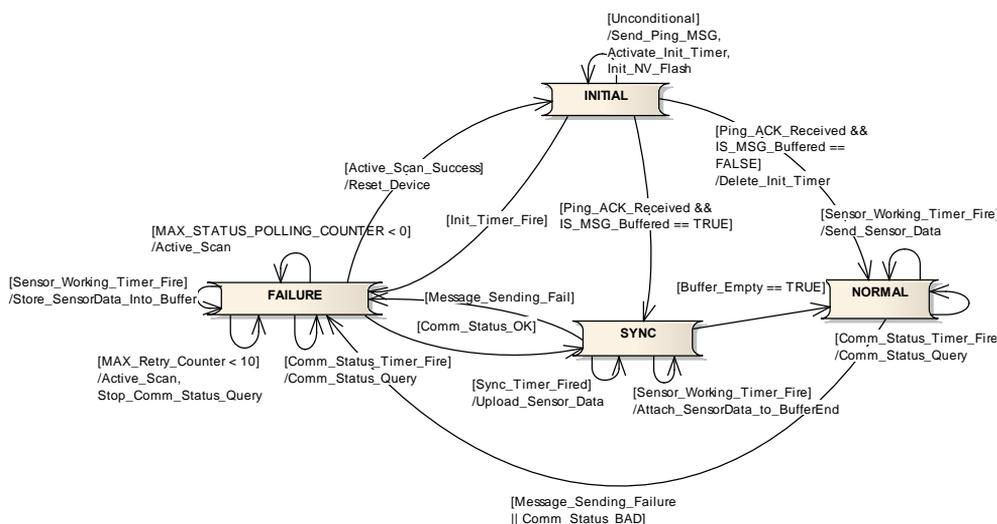
Fig.13 End device communication reliability enhancement state machine
