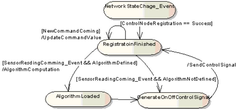
Fig. 12. Control node state machine
