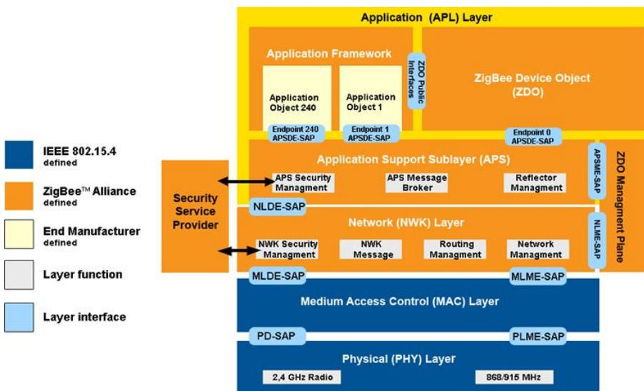
Fig.1 ZigBee software protocol architecture
