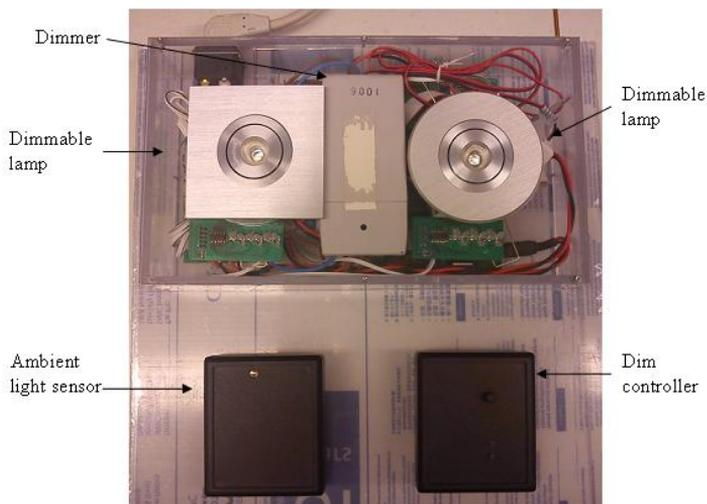
Fig.9 Dimmable lamp wireless control system
