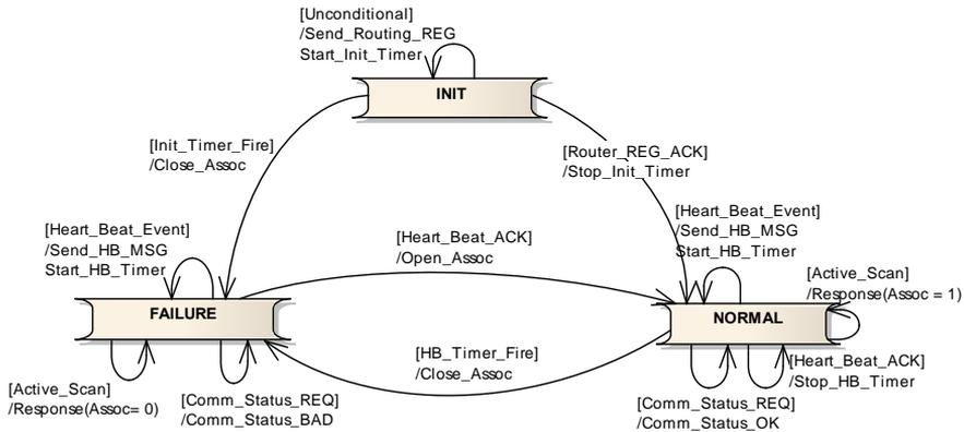
Fig.14 Router performance enhancement state machine
