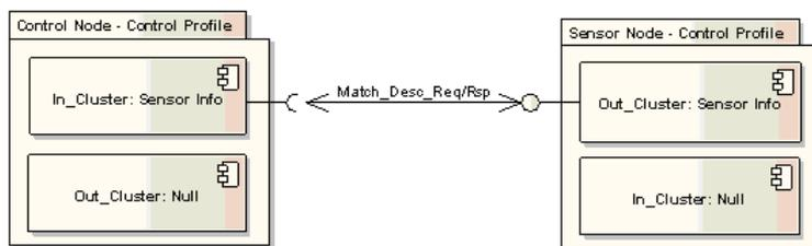
Fig. 11 Service discovery between the control node and the sensor node
