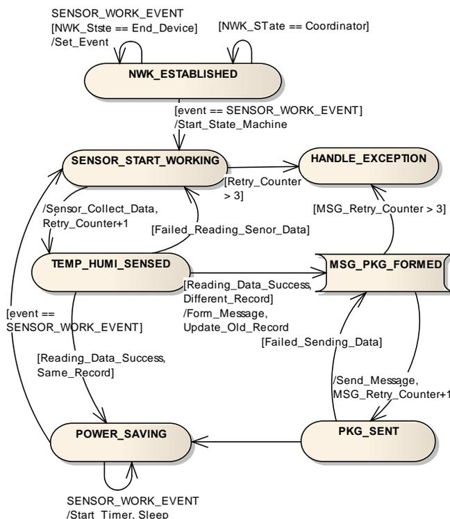
Fig.10 End device sensor operation state machine
