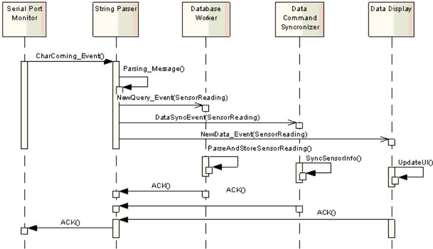
Fig. 16 Sensor information synchronization flow chart
