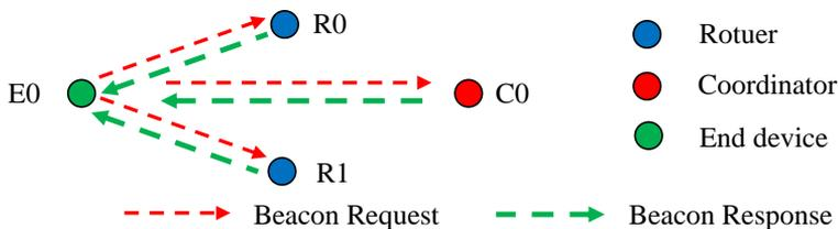
Fig.2 End device join the wireless sensor network via MAC association
