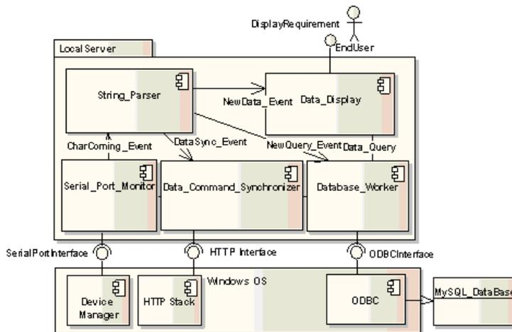
Fig. 15 Local server Software Architecture
