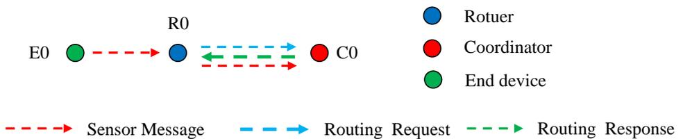
Fig. 3 ZigBee using AODV algorithm to create a new route
