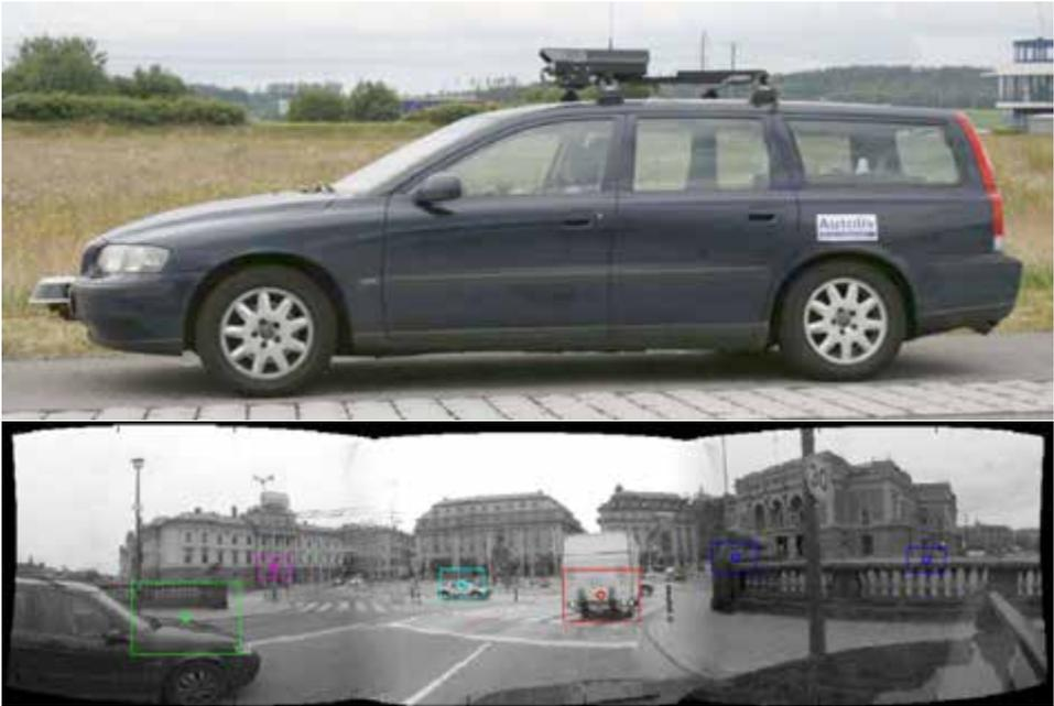
Figure 1.3: Top: The instrumented vehicle used in the DIPLECS project. Bottom: The combined view given by stitching the views given by the three individual cameras mounted on the roof of the vehicle.
