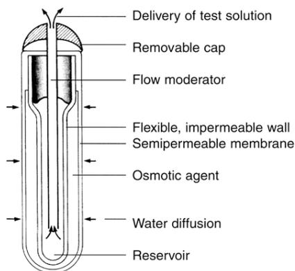
**Figure 8.** Schematic figure of an osmotic pump (adapted from Wamberg & Tauson, 1998).
