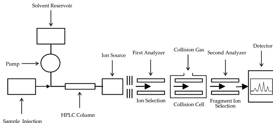
**Figure 6.** A schematic illustration of the LC-MS/MS instrumentation.
