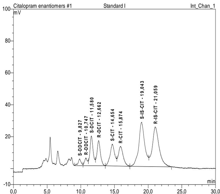
**Figure 9.** Representative chromatogram of a plasma standard sample prepared with concentrations of 31 nmol/l for the enantiomers of citalopram (CIT), 16 nmol/l for the enantiomers of demethylcitalopram (DCIT), and 3.5 nmol/l for the enantiomers of didemethylcitalopram (DDCIT).
