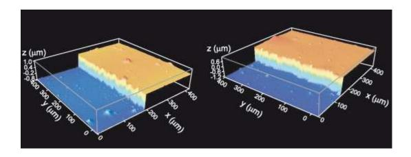
Figure 3. Images recorded by the optical profilometer provides the thicknesses of the PEDOT:PSS films.
