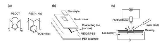
Figure 1. (a) Chemical structures of PEDOT and PSS (acid and sodium salt). (b) A drawing showing one of the EC display electrodes; two similar electrodes are then laminated to complete the EC display. (c) The experimental setup for the switching time measurement.
