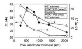
Figure 4. Color contrast ( $\Delta E^*$ ) and lightness (L\*) vs. the PEDOT:PSS thickness of the pixel electrode. Black filled circles represent  $\Delta E^*$ , while triangles and diamonds denote the L\* values of the white and colored state, respectively. A bias of +2.2 V and -1.2 V was used to obtain the electrochromic color switch between the fully reduced and the fully oxidized states. The inset shows the cross section image of the EC display used in this measurement.
