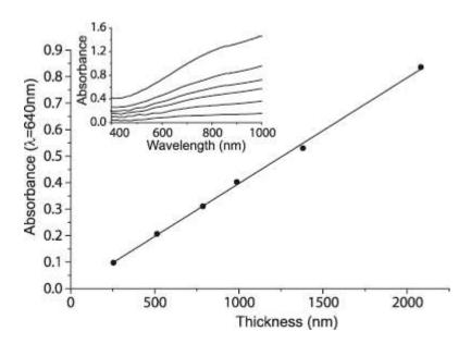
Figure 2. The absorbance vs. thickness dependence is illustrated, where the absorbance values were recorded at 640 nm. The inset shows the actual optical absorption spectra of the PEDOT:PSS coatings.
