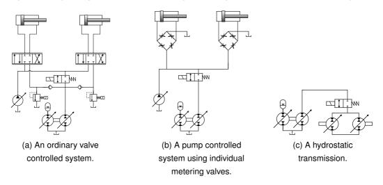
**Figure 3:** Examples of how the complementary energy recuperation system may be connected to standard hydraulic systems.
