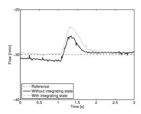
Figure 10: A step of 10% of the load pressure is made after 1 second.
