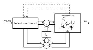
**Figure 4:** The proposed controller uses a feed forward gain on the reference signal based on the current working point of the system. The state feedback compensates for the dynamics of the system and reduces stationary errors due to model inaccuracies.
