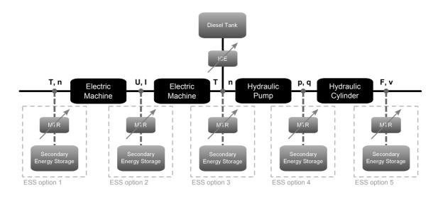
**Figure 1:** A stylized representation of a construction machine, demonstrating all possible connection nodes for a secondary energy storage system considering all possible domains present in the machine architecture.
