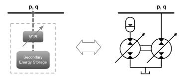
**Figure 2:** The hydro-mechanical transformer connected to a hydraulic node in the host system power flow, hence having a parallel structure.
