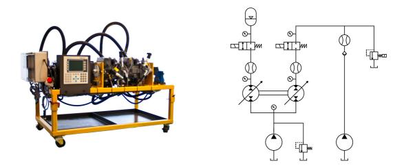
**Figure 7:** The hardware testbed is supplied with one pressure level for the low pressure side of the transformer and one controllable pressure level simulating the load pressure. The flow meters are used for model validation and analysis and not for control inputs.
