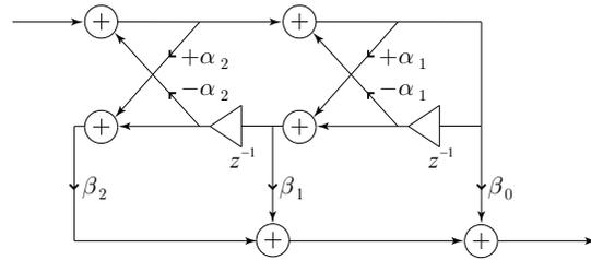
Figure 3: Lattice-ladder implementation of the scattering filter  $Q(z)$ .
