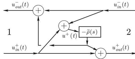
Figure 5: Displacement-wave scattering model for a spring.
