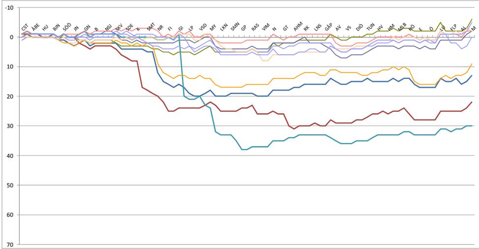
Figure 3. The X2000 service 521 and its deviation from its timetable at different locations along its journey from Stockholm (Cst) to Malmö (M). Statistics were collected during two weeks in October, 2010.
