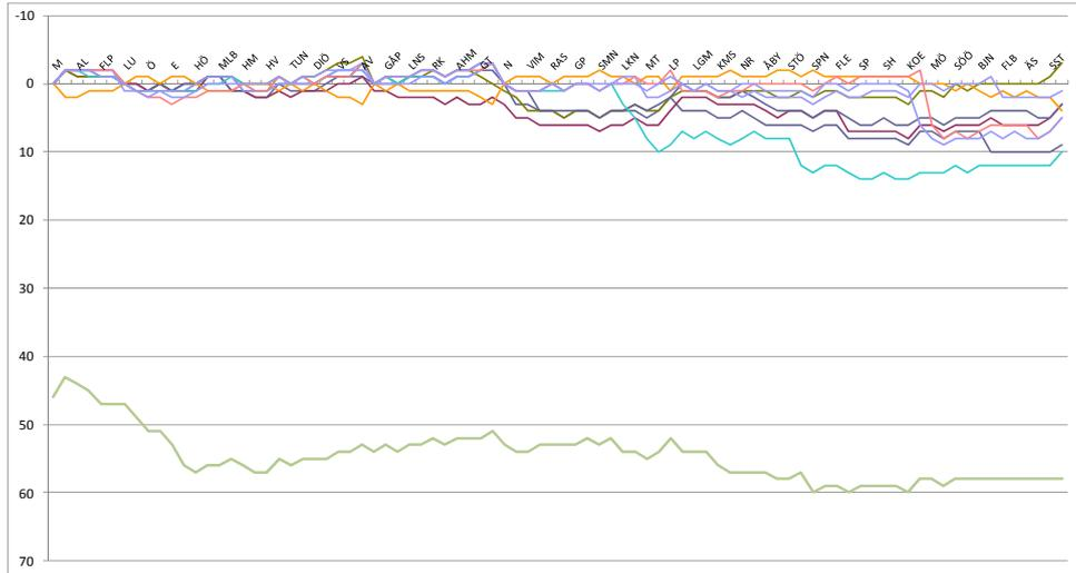
Figure 4. The X2000 service 524 and its deviation from its timetable at different locations along its journey from Malmö (M) to Stockholm (Cst). Statistics were collected during two weeks in October, 2010.
