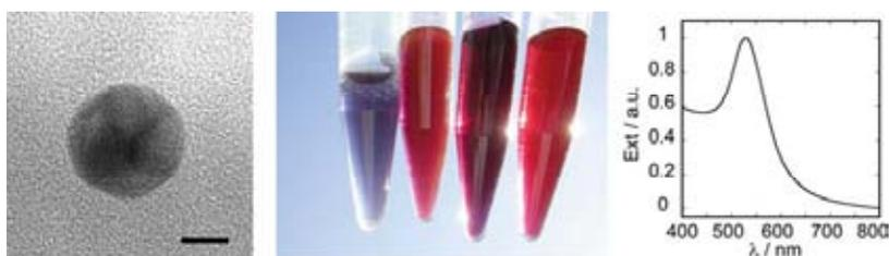
**Figure 5.1** (Left) Electron micrograph of a 13 nm gold nanoparticle (scale bar 5 nm), that are the cause of the beautiful colours of the dispersions in the photo in the middle. (Right) UV-visible spectrum of a dispersion of gold nanoparticles showing the characteristic extinction peak that gives rise to these colours. (Photo courtesy of Prof. M. Cortie, Institute for Nanoscale Technology, Sydney, Australia.)
