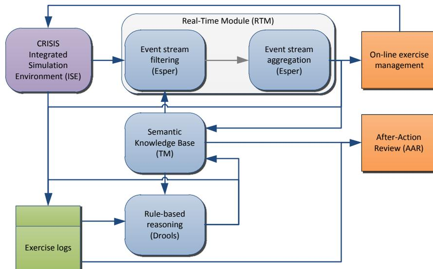
**Figure 1. The real-time situation assessment and decision support system (middle components) depicted within the context of the CRISIS system (leftmost components) and user modes (rightmost processes). The three main modules of the decision support system (DSS) are: Real-Time Module, Semantic Knowledge Base and Rule-Based Reasoning.**
