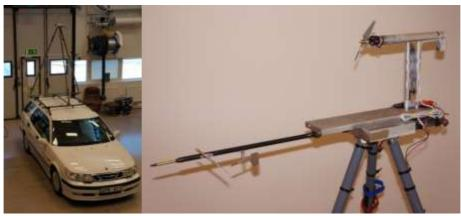
Figure 2. Car-mounted propeller test rig.
