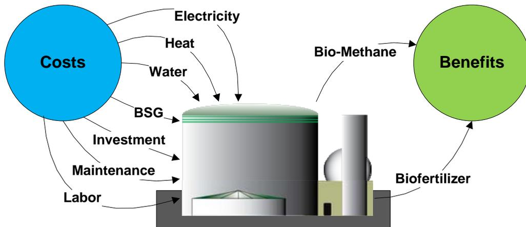
Figure 5. System boundary of the biogas plant applied in economic evaluation
