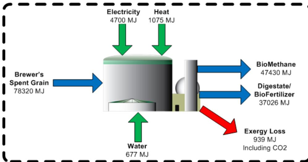
Figure 6. Exergy flow diagram of BIOLIU biogas plant
