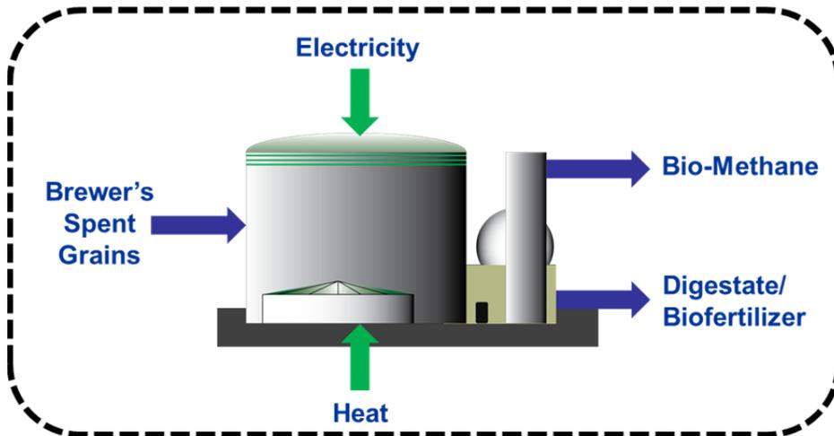
Figure 4: System boundaries of biogas production from BSG
