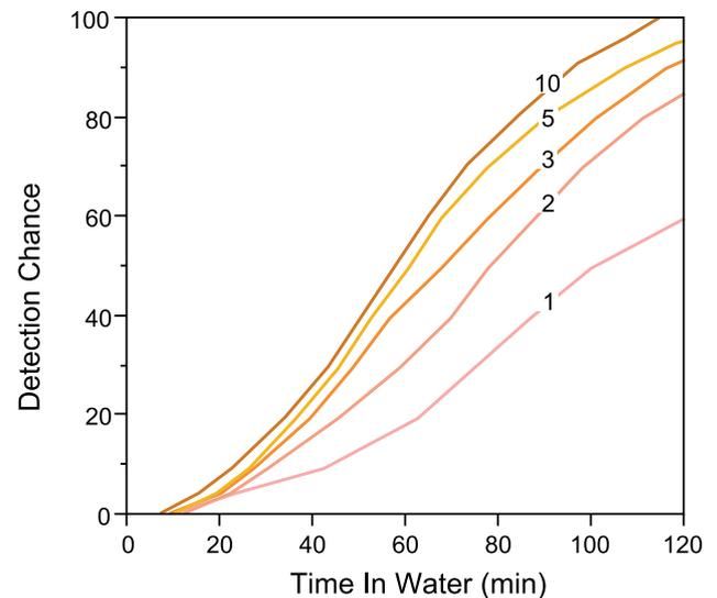
Fig. 7. Probability of detection versus time in the water for varying detection ranges for the baseline aircraft
