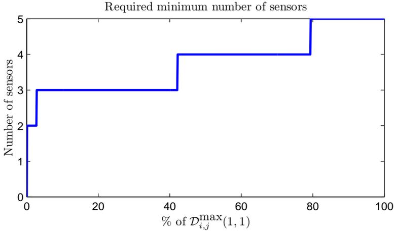
Figure 2: The least number of sensors required to exceed a certain percentage of maximum distinguishability given the example model (1). Note that the number of sensors when required performance goes to zero is equal to the cardinality of the minimal sensor sets (2) from the structural analysis.
