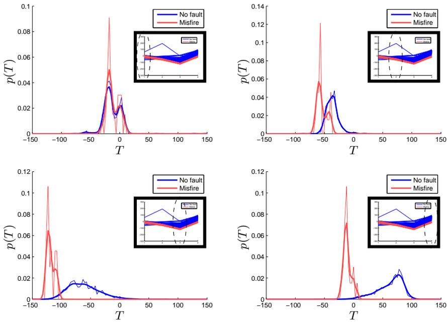
Figure 13: The distribution of the torque of cylinder 1, i.e., crank counts 1, 2, 3, and 4, during cold start at operating point speed 1500 rpm and load 1.2 g/rev. A normalized histogram of the data and an approximation of each distribution using kernels is shown in each plot. The separation between torque from fault-free combustion and a misfire is largest at the last sample and smallest at the first sample.
