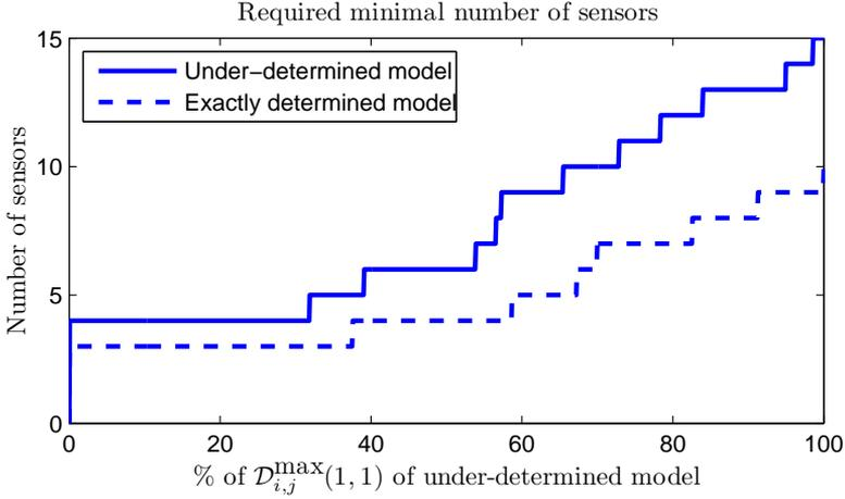
Figure 4: The least number of sensors required to exceed a certain percentage of maximum distinguishability given the underdetermined model described in Figure 3, for the underdetermined case and the exactly determined case, given a global search.
