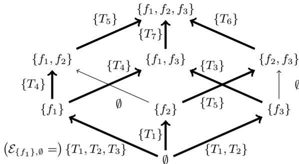
Figure 4: A lattice set representation of all possible candidates for a system with three possible faults. The set at each arrow represents which test quantities that are able to reject  $d_j$  for  $d_i$  and fulfills a specified distinguishability criteria.
