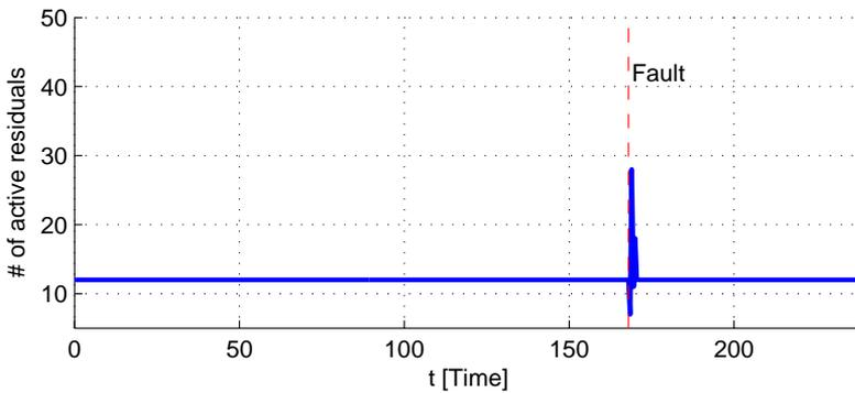
Figure 9: The number of active residuals during a scenario where two sensors fail,  $f_{24}$  and  $f_{35}$ , occurs at 168 s. The required minimum distinguishability for each residual is lower compared to the result in Figure 8 resulting in fewer active residuals during the scenario. The total number of active residuals during the scenario is 40.
