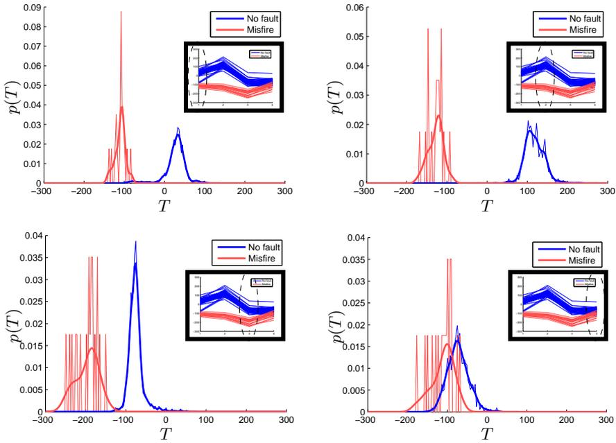
Figure 11: The distribution of the torque of cylinder 1, i.e., crank counts 1, 2, 3, and 4, during normal driving at operating point speed 1500 rpm and load 1.2 g/rev. A normalized histogram of the data and an approximation of each distribution using kernels is shown in each plot. The separation between torque from a fault-free combustion and a misfire is largest at the second sample and smallest at the last sample.
