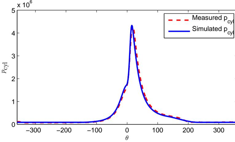
Figure 3: Cylinder pressure model compared to measurement data.
