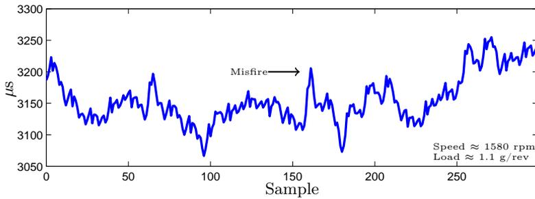
Figure 5: An example of the flywheel angular velocity signal from a six cylinder engine during cold start. Compared to signals in Figure 4, a misfire is more difficult to detect.
