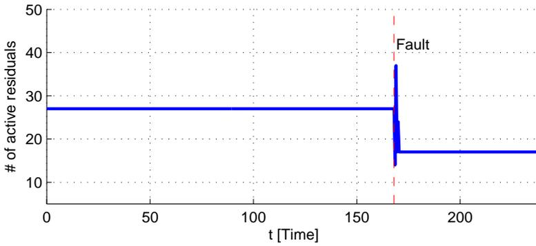
Figure 8: The number of active residuals during a scenario where two sensors fail,  $f_{24}$  and  $f_{35}$ , occurs at 168 s. The total number of active residuals during the scenario is 54.
