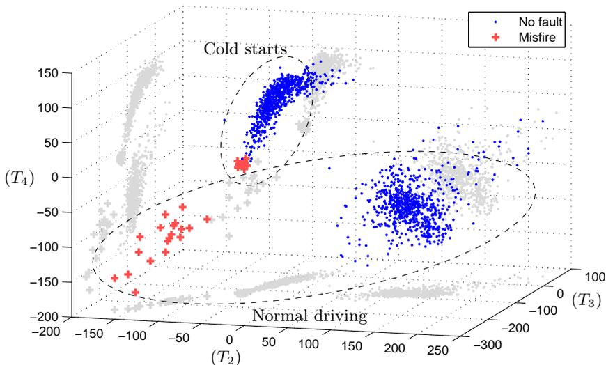
Figure 17: Estimated torque for three of the four samples shown in Figure 11 and Figure 13. The estimated torque at crank count 2 is  $T_2$ , the estimated torque at crank count 3 is  $T_3$ , and the estimated torque at crank count 4 is  $T_4$ .
