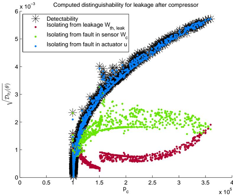
Figure 5: Computed distinguishability for a leakage after the compressor. Distinguishability for a leakage after the compressor from the no fault case, i.e., detectability performance, increases by increasing compressor pressure. Isolating the leakage from a leakage after the throttle, or a fault in the sensor measuring the mass flow through the compressor, affects the performance negatively while isolating from a fault in control signal  $u_\delta$  does not affect the performance noticeably.
