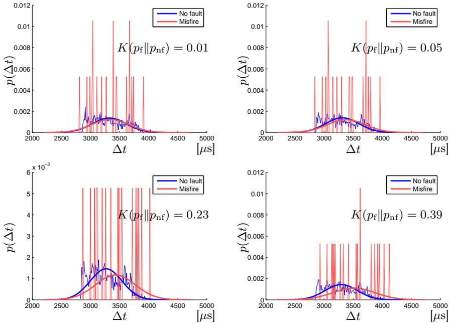
Figure 16: The distribution of the flywheel signal of cylinder 1 during normal driving at operating point speed 1500 rpm and load 1.2 g/rev. A normalized histogram of the data and an approximation of each distribution as a Gaussian is shown in each plot.
