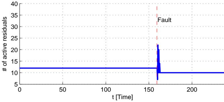
Figure 6: The number of active residuals during a scenario where a relay gets stuck open,  $f_{10}$ , occurs at 159 s. The required minimum distinguishability for each residual is lower compared to the result in Figure 5 resulting in fewer active residuals during the scenario. The total number of active residuals during the scenario is 41.
