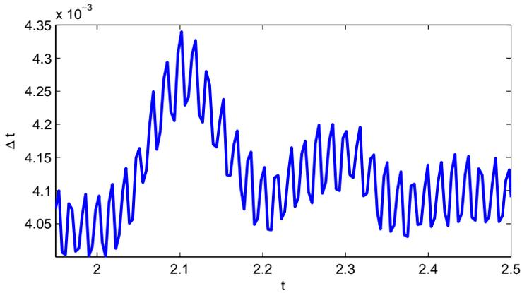
Figure 9: Simulated driveline disturbance at time 2 measured at the flywheel. Disturbance modeled as an impulse added to the constant required torque.
