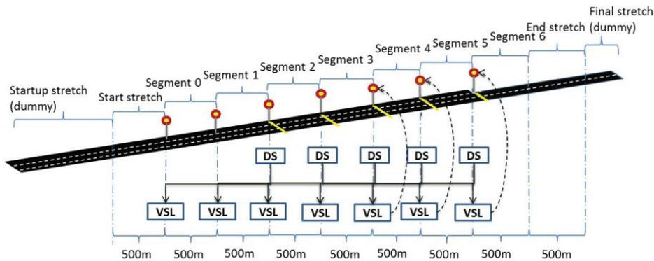
Fig. 2. Illustration of the considered VSLs and cooperative VSLs (VSL:Variable Speed Limit, DS:Detector System)
