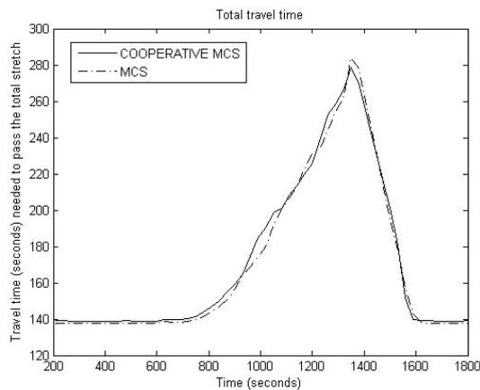
Fig. 6. Total mean travel time over the whole stretch based on 30 seconds intervals.
