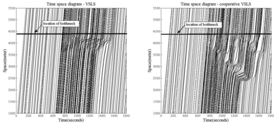
Fig. 3. Time-space diagram for the VLS and the cooperative VLS showing the trajectories for every fifth vehicle in the system (1 sec in update time for the cooperative VLS)
