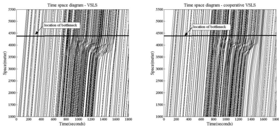
Fig. 4. Time-space diagram for the VLS and the cooperative VLS showing the trajectories for every fifth vehicle in the system (4 sec in update time for the cooperative VLS)
