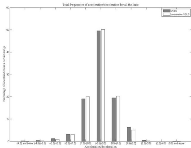
Fig. 5. Total frequencies of accelerations/decelerations rates (in percentage) of all links in the system for the VSLS and the cooperative VSLS
