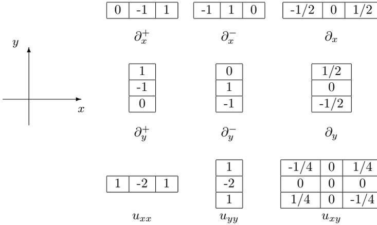
Figure 4.1: Convolution masks, where  $h = 1$  and the coordinate system on the left indicates the respective  $x$  and  $y$ -orientation.
