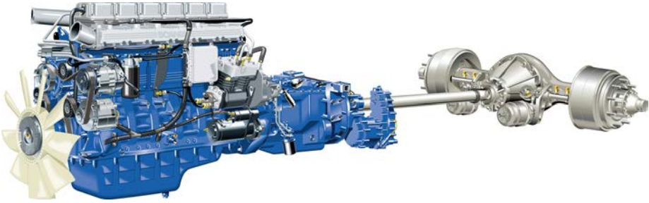
Figure 1.1: A rear-wheel-drive driveline from a Scania HDT. The engine, transmission, propeller shaft, differential (final drive) and drive shafts can be seen.
