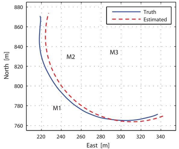
Fig. 7: Trajectory estimate of the all-terrain vehicle using the sensor network circular motion model (8); curved trajectory. M1, M2, M3 are the microphone positions. The estimate is compared to the ground truth.
