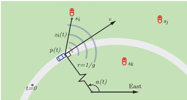
Fig. 2: Sensor network circular motion model. It is assumed that the source follows a circular trajectory  $p(t)$  with radius  $r = 1/g$ , where  $g$  is a model parameter that may take any value on the real axis. Model parameters are also the initial source location  $p_0 = p(0) = [p_x \ p_y]^T$  and origin angle  $\alpha_0 = \alpha(0)$ .
