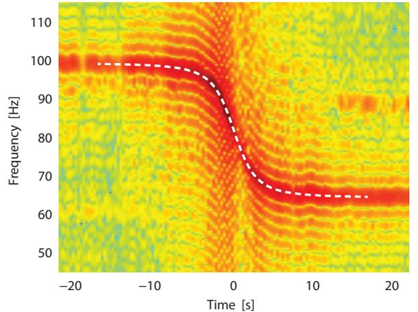
Fig. 4: Acoustic spectrogram of the Mooney M20J passing 220 m from the sensor at 73 m/s. The white dashed line is the frequency according to the identified model (3) combined with (5).  $t = 0$  is the true passage time (closest point of approach) according to the GNSS receiver.
