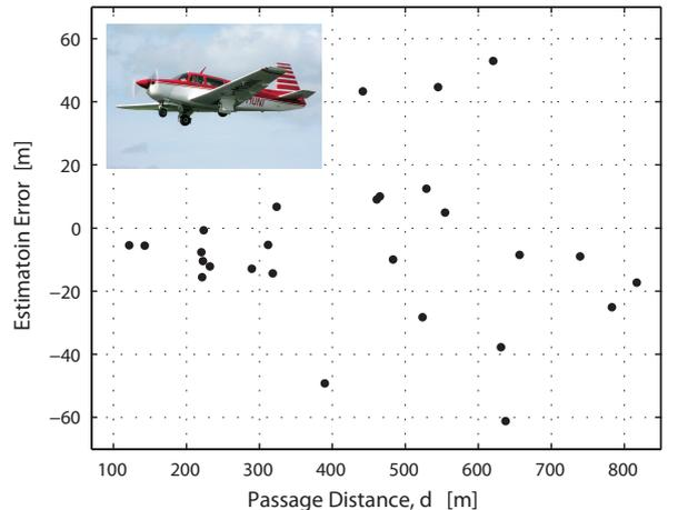
Fig. 5: Distance error versus distance for 28 passages of a Mooney M20J aircraft.
