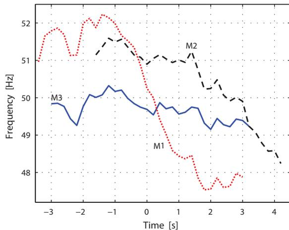
Fig. 8: Frequency estimates used as input to the model identification in Fig. 7. The fundamental source frequency is apparently around 50 Hz. The Doppler shift is clearly manifested, although the noise level is high with respect to the shift.
