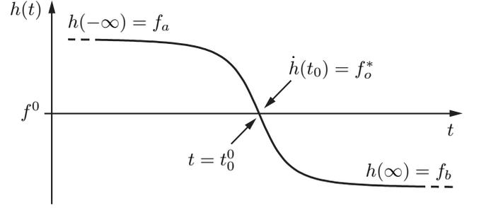
Fig. 3: Features extracted for the initial estimate for the single sensor linear motion model. The key features are the asymptotic frequencies,  $f_a$ ,  $f_b$ , and the slope of the frequency curve at the closest point of approach,  $f_o^*$ .
