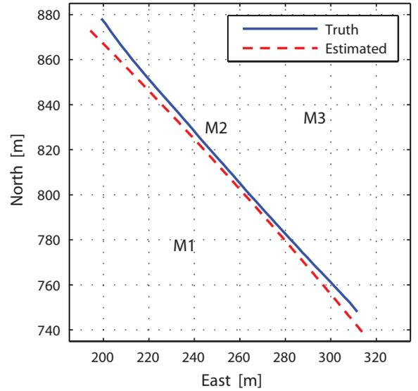
Fig. 6: Trajectory estimate of the all-terrain vehicle using the sensor network circular motion model (8); straight trajectory. M1, M2, M3 are the microphone positions. The estimate is compared to the ground truth.
