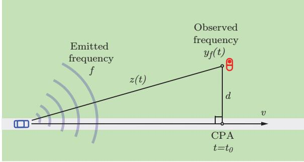
Fig. 1: Single sensor linear motion model. It is assumed that the source, here illustrated by a car on a road, moves along a straight line at constant speed  $v$  emitting a constant frequency  $f$ . At  $t = t_0$  the source attains its closest point of approach (CPA) with respect to the observer, for instance the microphone.  $z(t)$  is the source-observer distance. The object is to determine  $d$  and  $v$  by observing the Doppler variations in the received frequency  $y_f(t)$ .
