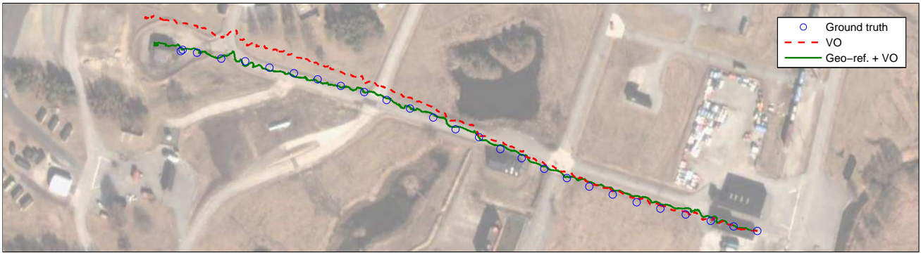
Fig. 6. True trajectory illustrated with circles and the estimated trajectories with (solid line) and without (dashed line) geo-referencing.
