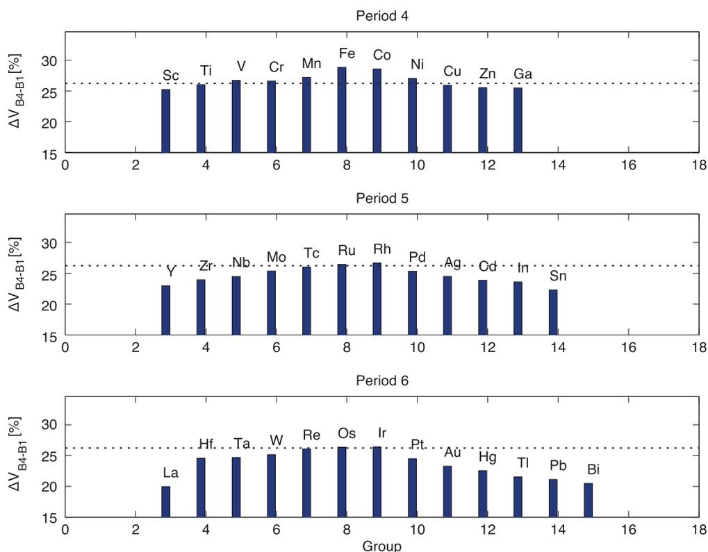
**Figure 5.** Relative difference in volume  $\Delta V_{B4-B1}$  between B1 and B4 crystal structure of AlN doped with TM impurities. AlN relative volume difference is shown as reference by the dotted line.
