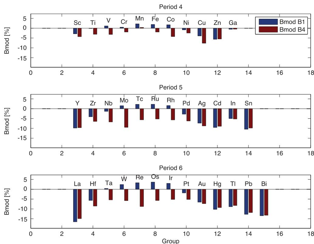
**Figure 7.** Change in bulk moduli of B1 (blue) and B4 (red) AlN doped with TM impurities relative to stoichiometric AlN. Calculated in the same way as  $\Delta V_{\text{alloy}}$  above, but for bulk modulus instead of volume.
