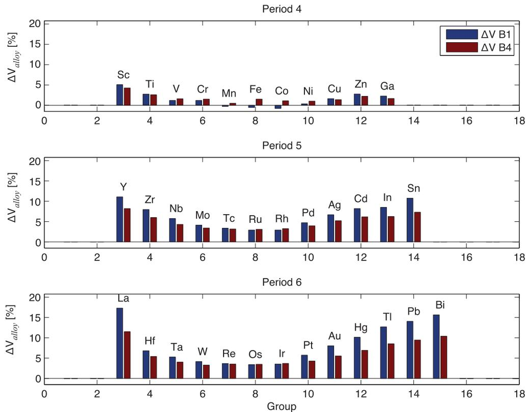
**Figure 4.** Change in volume  $\Delta V_{\text{alloy}}$  for B1 (blue) and B4 (red) AlN doped with TM impurities relative to stoichiometric AlN.
