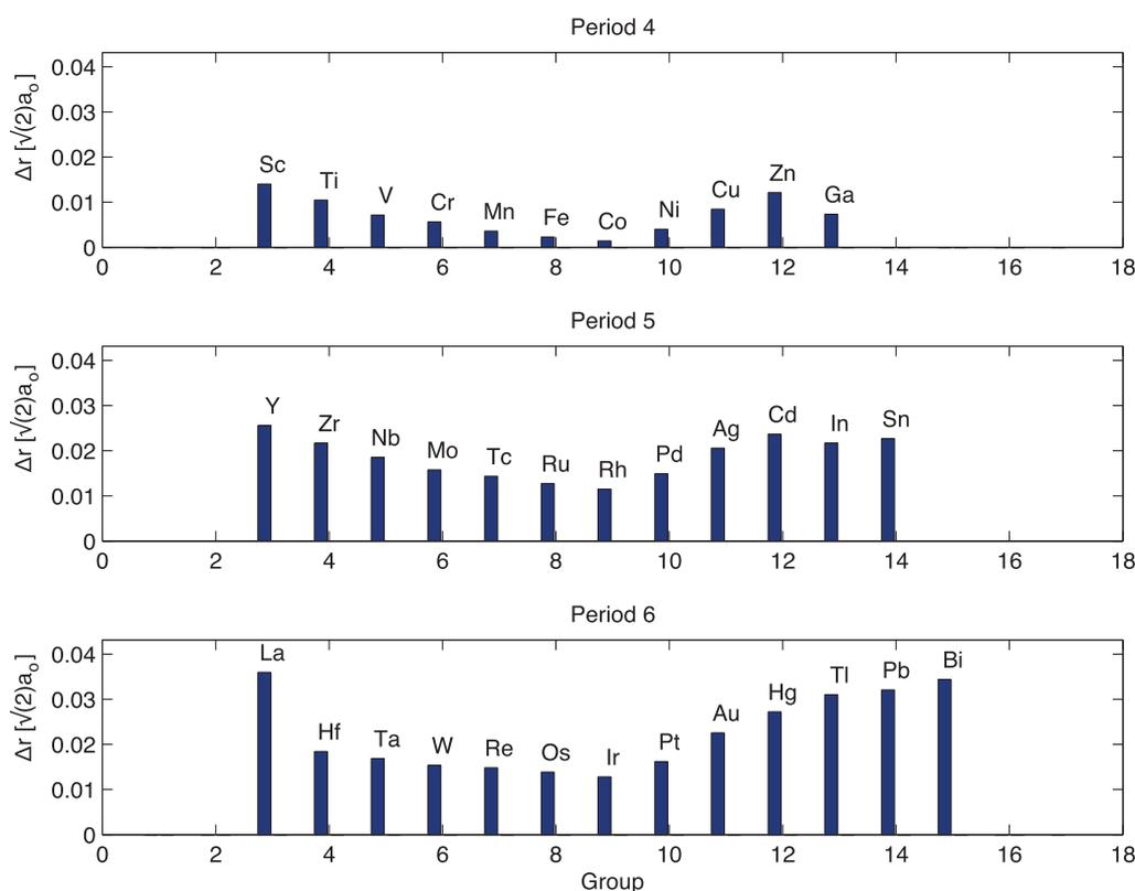
**Figure 8.** Deviation of N-atoms positions from the ideal crystal coordinates in B1 crystal structure, given in units of the basis vector length  $\sqrt{2}a_0$  where  $a_0$  is the fcc lattice parameter for the given alloy.
