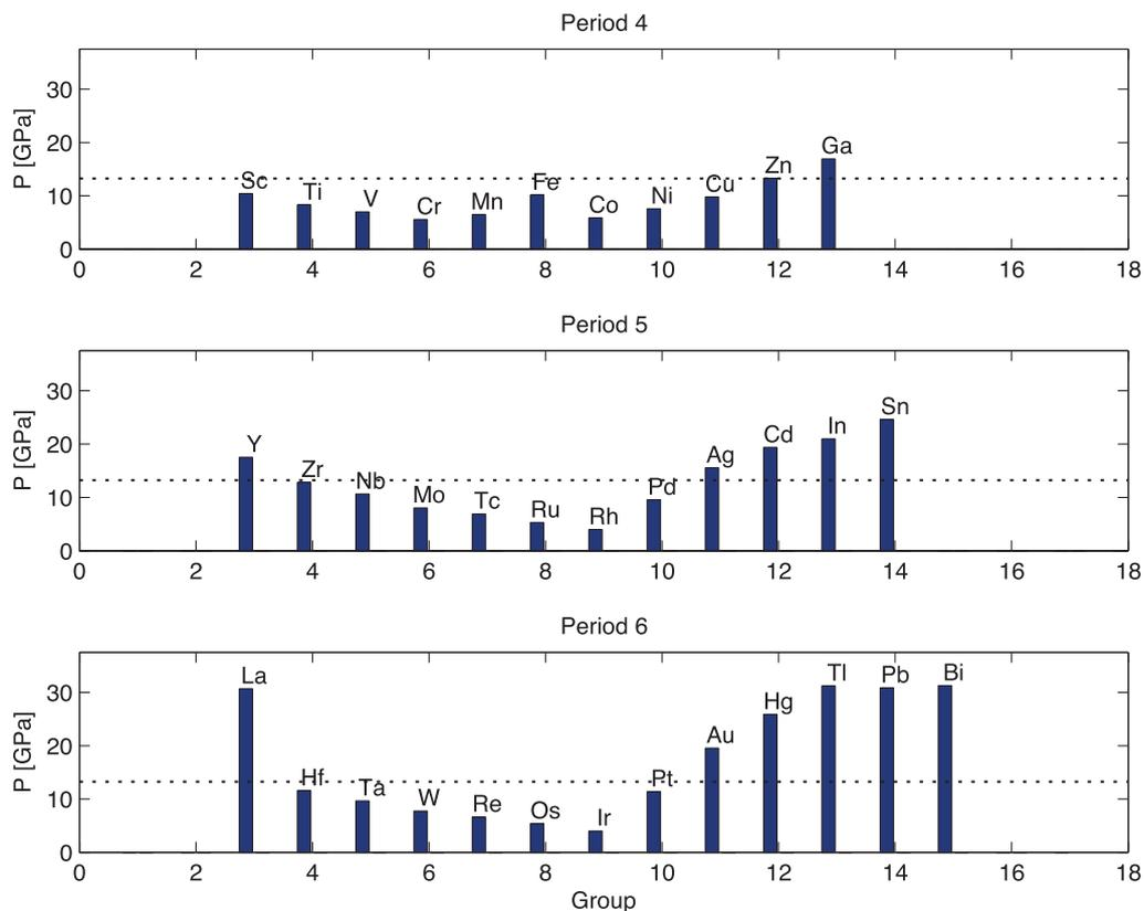
**Figure 6.** Zero temperature values of pressure  $P$  for B4–B1 phase transformation in AlN doped with TM impurities. The transition pressure for pure AlN is marked as a dotted line for reference.
