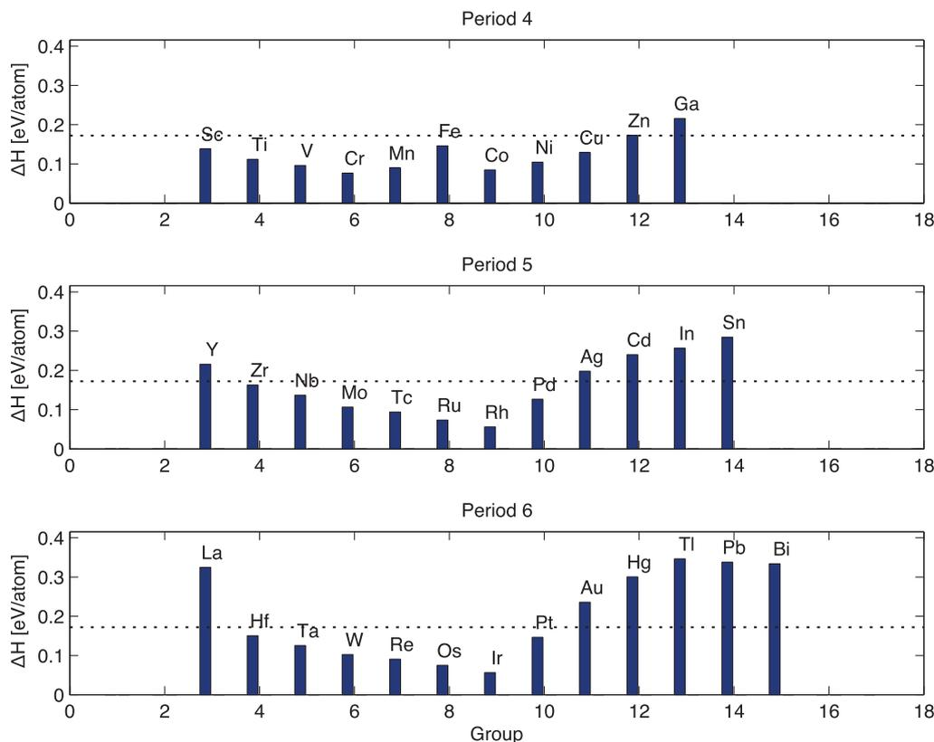
**Figure 3.** Variation of the enthalpy difference at zero pressure  $\Delta H_{B1-B4}$  equation (1), between B1 cubic and B4 wurtzite phases of doped AlN with the position of the impurity atom in the TM series. The dotted line shows pure AlN as reference. A clear trend is seen where the TMs in the middle of the periodic table, groups 6–9, iron being an exception, show a marked decrease in the enthalpy difference between the two structures.
