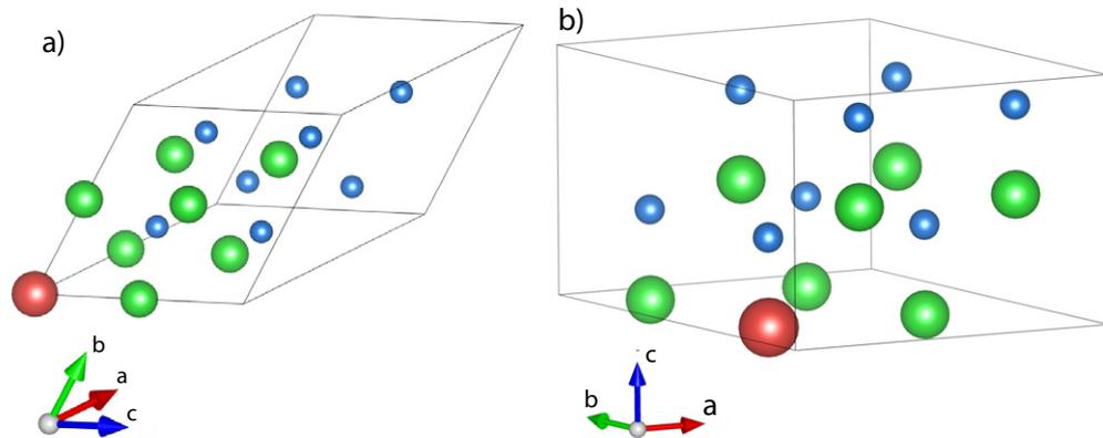
**Figure 1.** Schematic representations of the model structures used in the calculations. A B1  $2 \times 2 \times 2$  cell is seen in (a) and a B4  $2 \times 2 \times 1$  cell is seen in (b). Blue spheres are N-atoms, green are Al and red is the metal impurity atom.
