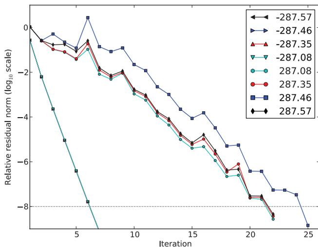
FIG. 2. Relative residual norm versus number of CC-CPP solver iterations to obtain the response amplitudes  $t^X(\omega + i\gamma)$  at chosen frequencies (given in the legend). The value of the damping parameter is  $\gamma = 1000 \text{ cm}^{-1}$ . The relative threshold of convergence at  $10^{-8}$  is indicated by a horizontal line. Note that the trend lines of the four negative frequencies (converging in 7 iterations) overlap completely.
