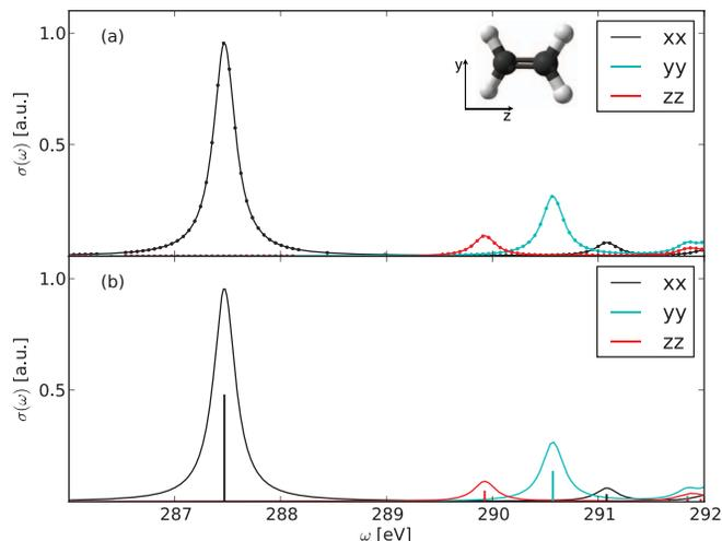
FIG. 1. NEXAFS spectrum [xx- (black), yy- (red), and zz- (blue) component] of ethene at the CCSD level obtained with the (a) CC-CPP and (b) Lanczos-based solver. Lanczos chain length is 4000,  $\gamma = 1000 \text{ cm}^{-1}$ , and threshold is  $10^{-8}$ .
