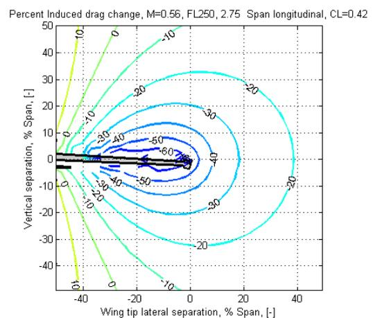
**Fig 7: Iso curves of induced drag reduction from the numerical simulation.**
