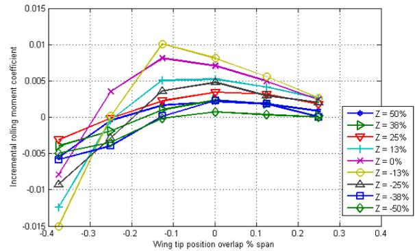
**Fig 10: Incremental rolling moment coefficient at different wing tip overlaps and height offset, numerical results.**
