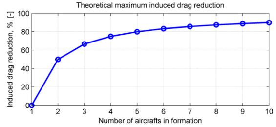
**Fig. 1 Expected theoretical maximum induced drag reduction from formation flight, based on increased virtual aspect ratio.**
