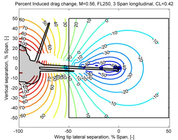
**Fig 6: Iso curves of induced drag reduction., showing the F/A 18 outline.**
