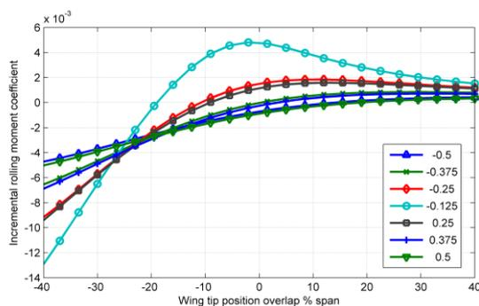
**Fig 9: Incremental rolling moment coefficient at different wing tip overlaps and height offset, numerical results.**
