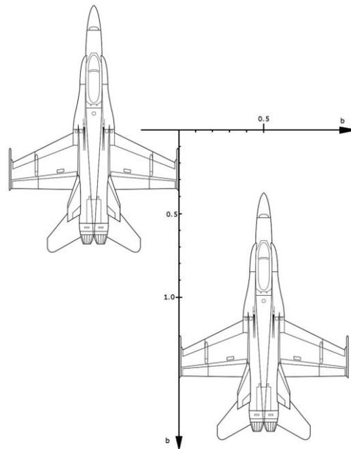
**Fig. 2 Coordinate system. When the aircraft are line abreast, wing tips touching, they are at origin position [0 0 0].**
