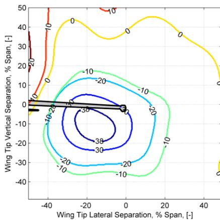
**Fig 8: Iso curves of induced drag reduction from NASA flight tests.**
