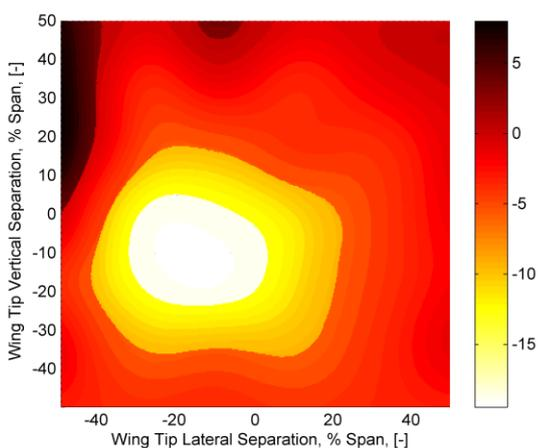
Fig 3: Overall drag reduction. in %, as a function of wingtip separation as reported by [3].
