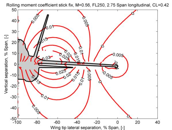
**Fig 11: Incremental rolling moment coefficient**
