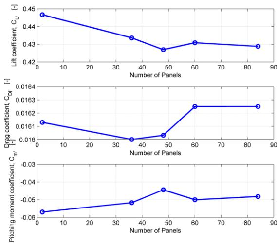
**Fig 5: Grid convergence history. Number of panels in the entire geometry.**
