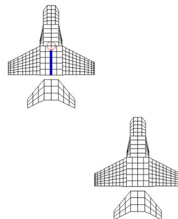
Fig 4: Mesh distribution of the numerical simulation with the following aircraft in position [1.3 0 0].
