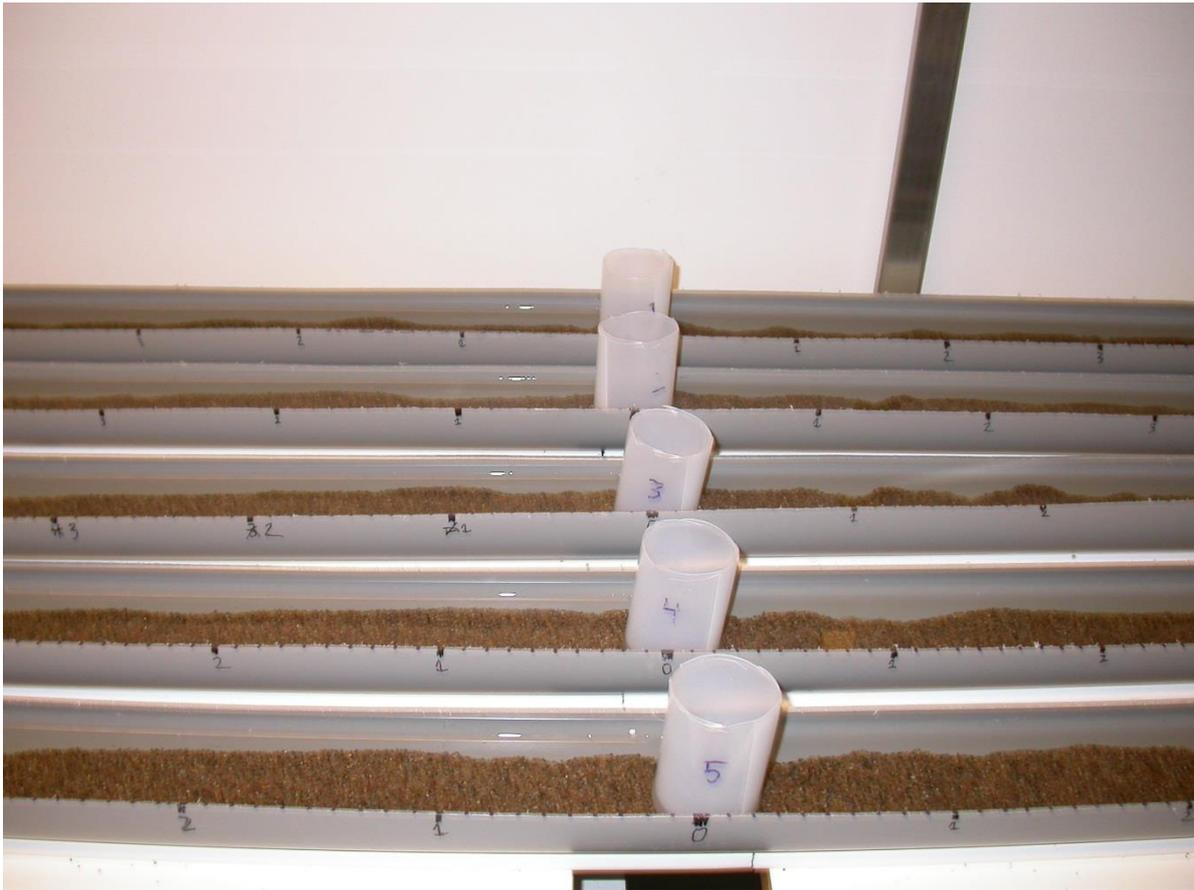
Figure 1 *Five experimental halfpipes were used for the test runs, filled with Rådasand and water from Lake Tåkern. Cylinders made from polypropylene bottles were used as containers for the test animals before each run.*
