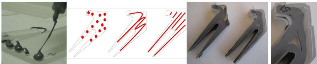
**Figure 5.** To the left are a picture of an adhesive string and illustrations of different patterns for the application of adhesive; to the right, two pictures showing air trapped between joined blocks.
