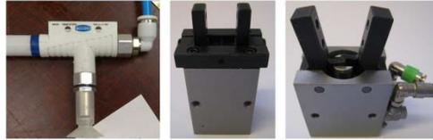
**Figure 1.** A vacuum cup with an ejector system (left). Two examples of clamping grippers (right).
