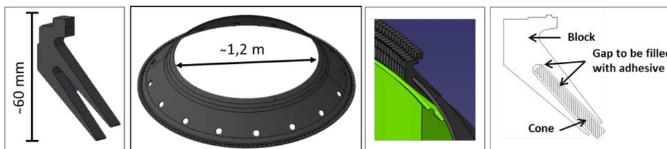
**Figure 2.** The two leftmost illustrations are a 3D CAD representation of the block and a picture of the truncated cone, while the two illustrations to the right show how a block is assembled on the cone.
