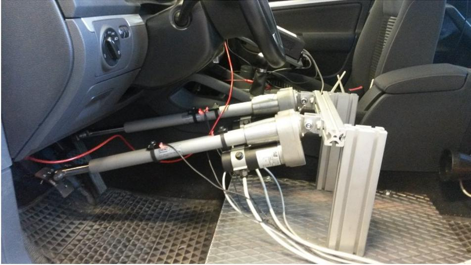
**Figure 2.7:** Pedal robot mounted in a vehicle instead of the driver's seat. The actuators are connected to the gas and clutch pedals. The red cable in the figure is from the OBD reader tool connected to the vehicle's OBD port.
