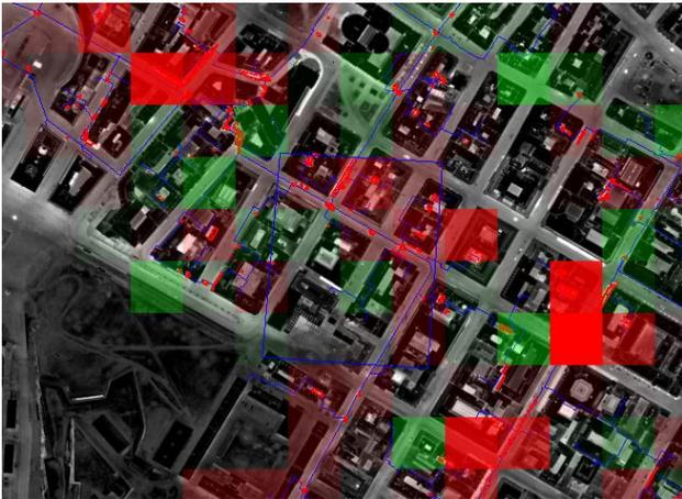
Fig. 7 Visualization of changes in radiated power. A red square indicates that the area suffers from an increased energy loss while a green square means that the energy loss within the area has decreased.
