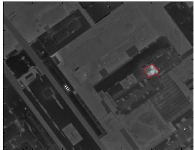
Fig. 9 Example of a false detection (marked with red boundaries) that has been removed with the help of a building mask.
