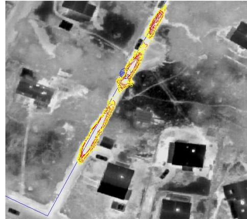
Fig. 3 Example of visualization of two layers of detections (red and yellow lines). The blue line is the district heating network.
