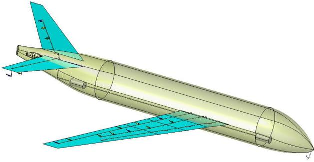
Figure 11: Final flight control assembly integrated in RAPID.
