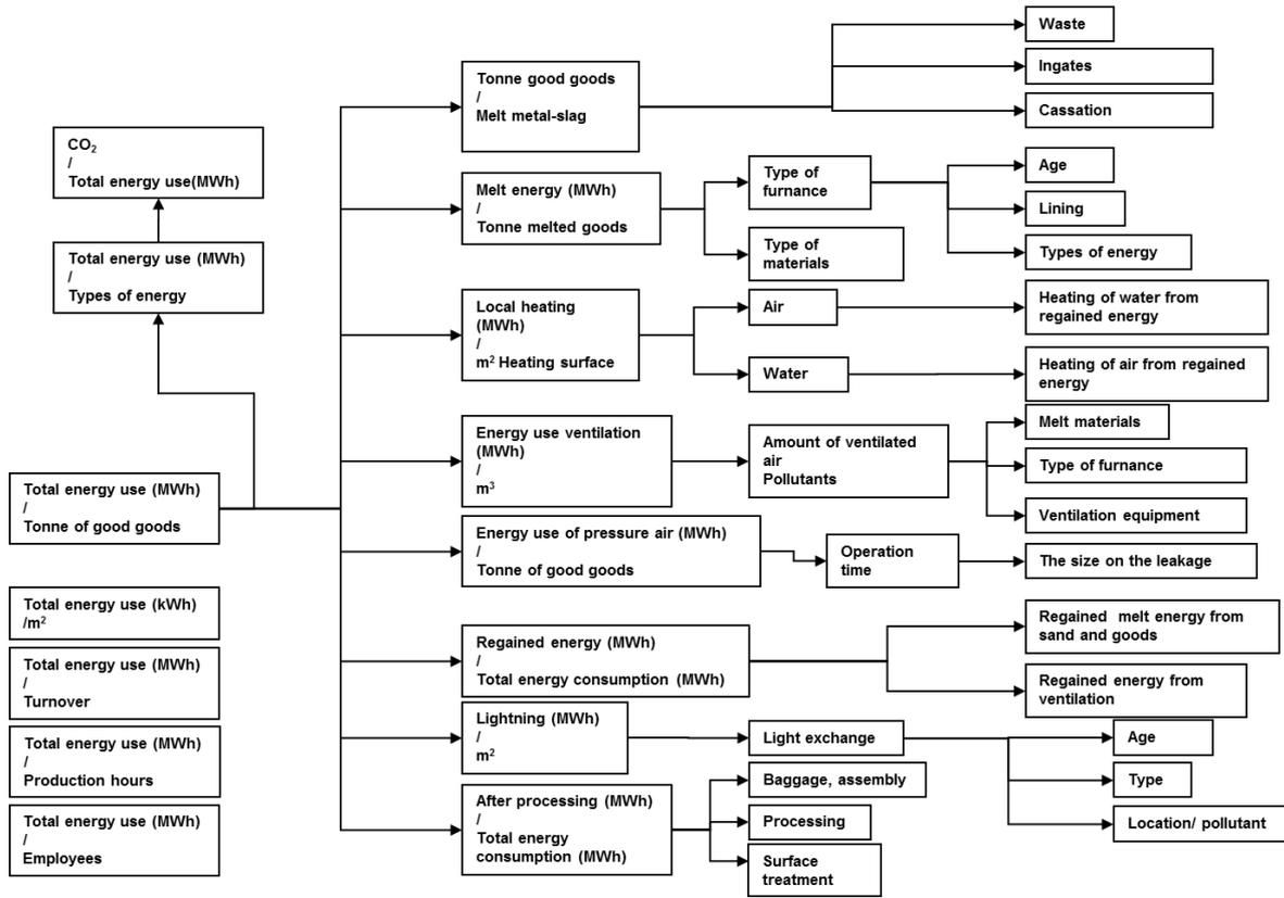
Figure 3- Above is an example on how energy relevant KPIs are related to each other in a sand-mould foundry.
