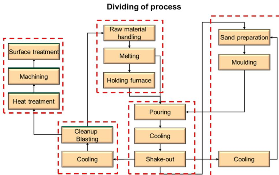
Figure 1- Division of processes in sand-mould foundry
