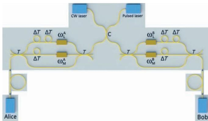
**Fig. 5. Experimental setup of the attack on the Franson interferometer.** The source consists of a CW laser for blinding the detectors, a pulsed laser for generating the bright classical light pulses, fiber optic couplers (C) delay loops ( $\Delta T$ ), phase modulators ( $\omega$  and  $\phi$ ), and detectors (D). Alice and Bob have the same analysis stations as in Fig. 1.
