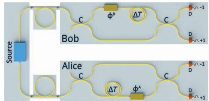
**Fig. 1. Experimental setup of the Franson interferometer.** The setup consists of a source,  $2 \times 2$  couplers (C), delay loops ( $\Delta T$ ), phase modulators  $\phi^A$  and  $\phi^B$ , and detectors (D).
