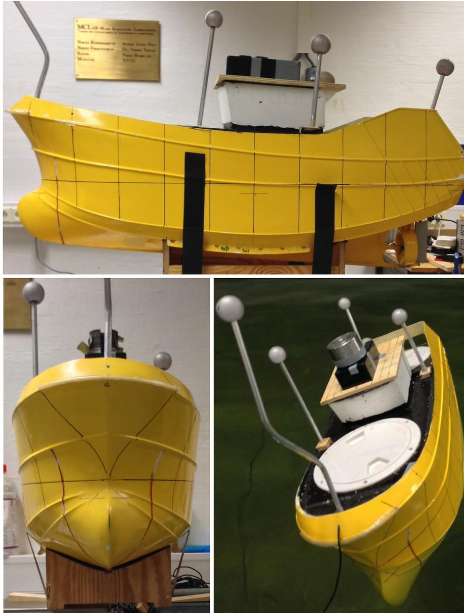
Figure 3: Top: A side view of the scale model that was used in the experiments. The IMU was located underneath the black and gray box on the top. Left: The ship seen from the front. Note that the change in wetted surface due to a roll motion should be small since the ship is square in shape. Right: The ship was very sensitive to the loading condition. The picture shows the massive roll angle resulting from a load mass of 2 kg corresponding to a 9% increase in mass.
