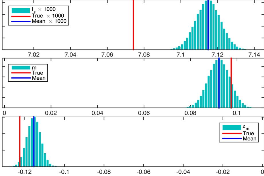
Figure 6: The result from the estimation of the parameters in Table 1. Here, only the parameters with known true values are shown. Red corresponds to the measured or calculated physical quantity in Table 1. Cyan is the histogram of the samples drawn from  $\mathcal{N}(\hat{\vartheta}, \hat{P}_\vartheta)$  and blue corresponds to the the sample mean. Top:  $I_x$ , middle:  $m$  and bottom:  $z_m$ .
