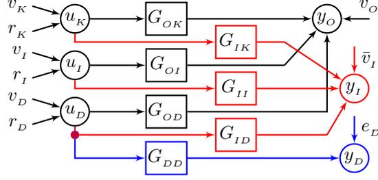
Figure 2: The model (5) seen as a dynamic network where circle corresponds to sums and blocks corresponds to the transfer functions. The black parts corresponds to the model of interest, red corresponds the indirect input measurements and blue corresponds to the direct input measurements.
