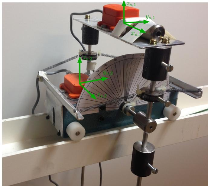
Figure 5: A picture of the modified inverted pendulum. Uppermost in the picture is the IMU (orange) measuring the rolling motion. In front of it is the additional load fastened with white tape. To the left on the cart is the reference IMU.
