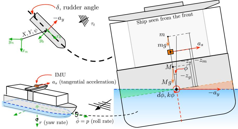
Figure 4: A sketch of a ship performing a turning maneuver which results in an unknown acceleration  $a_y$  acting on the CR. The shift in displaced water (green/red area) forces the ship back towards its equilibrium.
