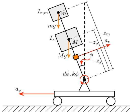
Figure 3: A sketch of the approximate inverted pendulum model showing the relation of the important quantities.
