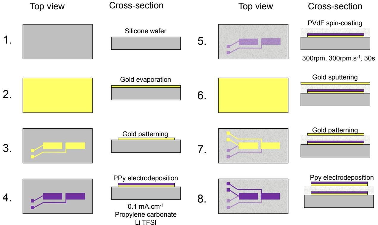
Fig 2: Process flow of the bottom-up microfabrication of tri-layer actuators.
