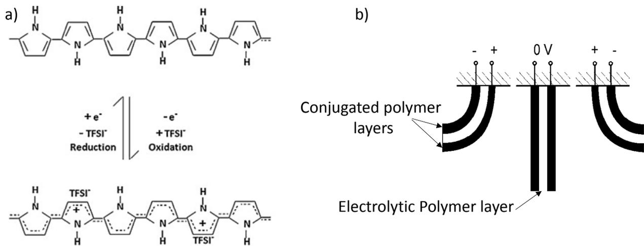
Figure 1: a) Oxidation-reduction process of the conjugated polymer and illustration of the bending of a trilayer conjugated polymer actuator
