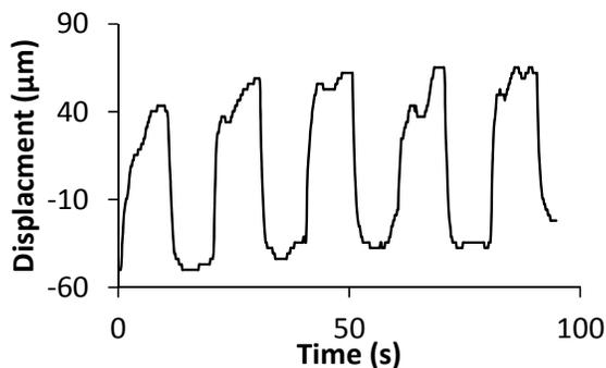
Fig 4 Tip displacement of the top actuator under an application of  $\pm 1 \text{ V}$  at  $0.05 \text{ Hz}$ .
