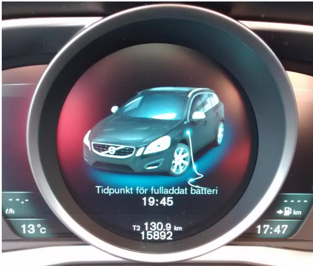
Figure 5: The Volvo V60 PHEV charging and showing an estimation of when the battery will be fully charged in the dashboard.
