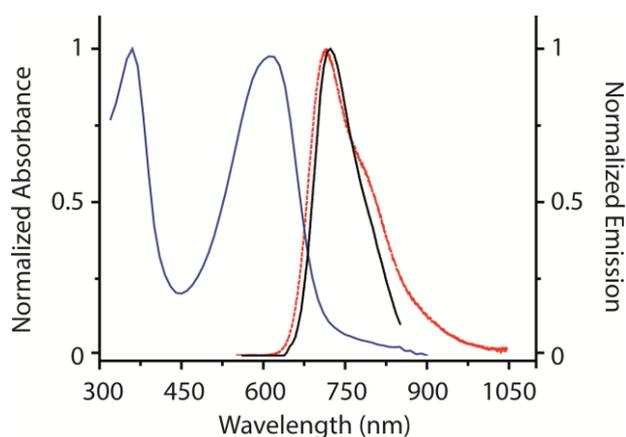
**Figure 2.** Normalized absorbance (blue, solid) and fluorescence emission spectra of TQ1 thin films excited at 533 nm (red, dashed). The absorbance spectrum shows maxima at 360 nm and 620 nm and the fluorescence emission appears at about 720 nm. Emission spectrum from a single TQ1 fiber (black, solid) obtained using wide-field spectral imaging show an emission maximum at about 730 nm.
