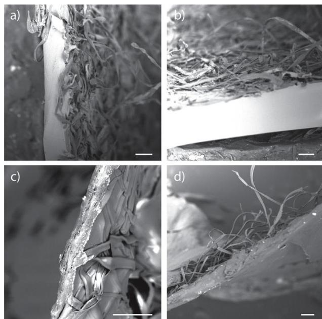
**Figure 3.** Scanning electron micrographs of electrospun TQ1 fibers physisorbed on a), b) PDMS and c), d) collagen hydrogel substrates. Scale bars: 50  $\mu\text{m}$ .
