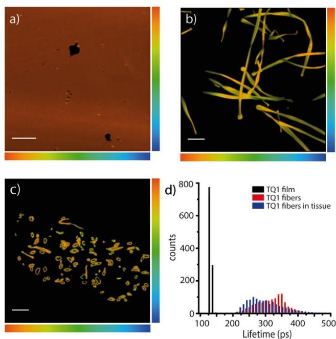
**Figure 7.** Fluorescent lifetime images a) a thin spun-coated film of TQ1 on a glass substrate, b) electrospun TQ1 fibers on a glass substrate and c) TQ1 fibers in tissue. Color bar denotes the fluorescent lifetimes from 100 ps (orange) to 110 ns (blue). d) Histogram showing the distribution of fluorescence decays for TQ1 film (black), TQ1 fibers on glass (blue) and TQ1 fibers in tissue (red).
