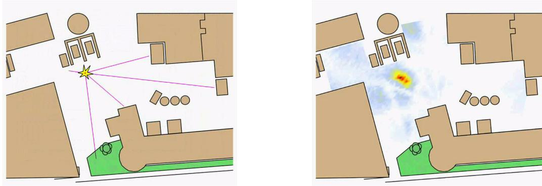
Figure 3. Localization using acoustic sensors. Left: Gunfire. Right: A shouting mob.
