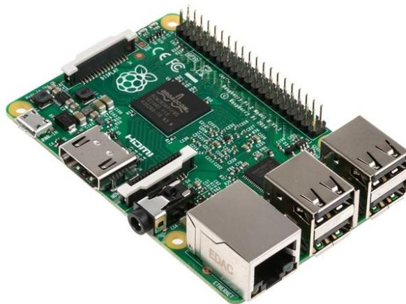
Figure 4: A Raspberry Pi 2 (Element14.com, 2015).
