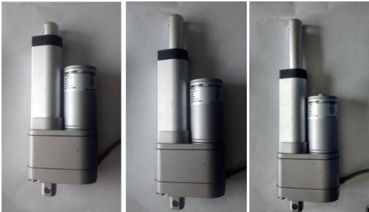
Figure 19: Potentiometer Values: 50 (L), 512 (M), 980 (R) representing different absolute positions of the actuator.
