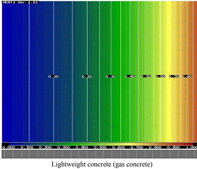
Figure B4a. Temperature profile in a cross-section of wall segment with lightweight concrete after 8 hours charging with 1°C.
