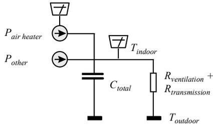
Figure 5.2. Electrical analogy model of the Övertorneå test house.
