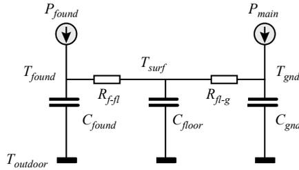
Figure 5.8. Simplified electrical analogy model of the Hus 15 test house.
