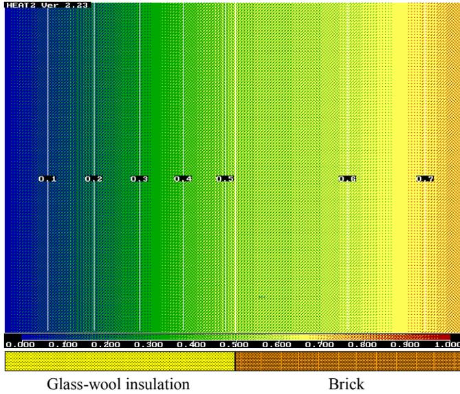
Figure B3a. Temperature profile in a cross-section of wall segment with brick and glass-wool insulation on the outside after 8 hours charging with 1°C.
