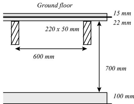
Figure 5.7. Crawl-space foundation.
