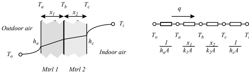
Figure 4.6. Physical model and electronic circuit model of overall heat transfer through a plane wall.
