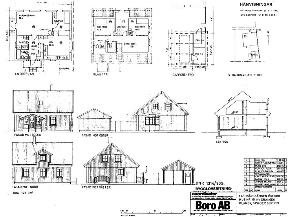
Figure C3. Face and plan of the Hus 15 test house.
