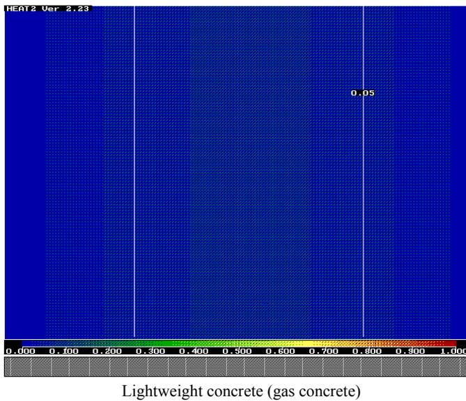
Figure B4b. Temperature profile in a cross-section of wall segment with lightweight concrete after 16 hours discharging with 0°C.
