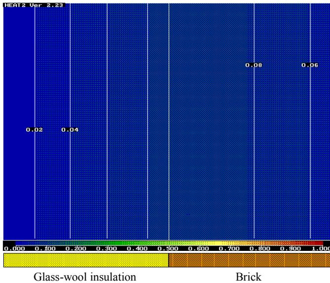
Figure B3b. Temperature profile in a cross-section of wall segment with brick and glass-wool insulation on the outside after 16 hours discharging with 0°C.
