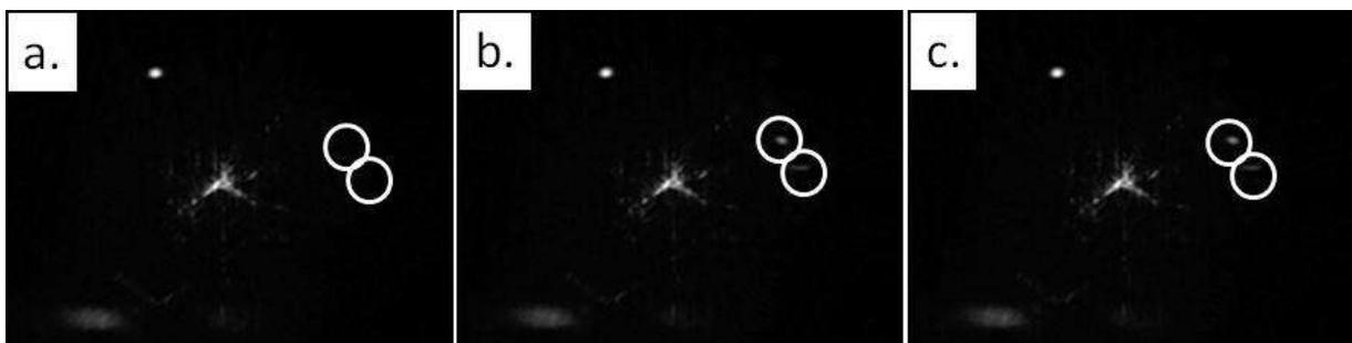
Figure 6: iSPR images demonstrating a touchdown event on a MUDA surface. The image sequence shows the occurrences of the touchdown events which were not observable (a) before the event, (b) occurred for a short period of time (marked with a white circle) and (c) remained there after initial touchdown, leaving an organic material behind.
