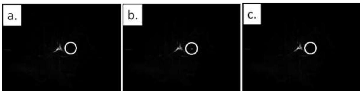
Figure 4: iSPR images demonstrating a touchdown event on an mPEG surface. The image sequence shows the occurrences of a touchdown event which was not observable (a) before the event, (b) occurred for a short period of time (marked with a white circle) and (c) disappeared after the event. The triangular spot in the center of the images is a reflection artefact.
