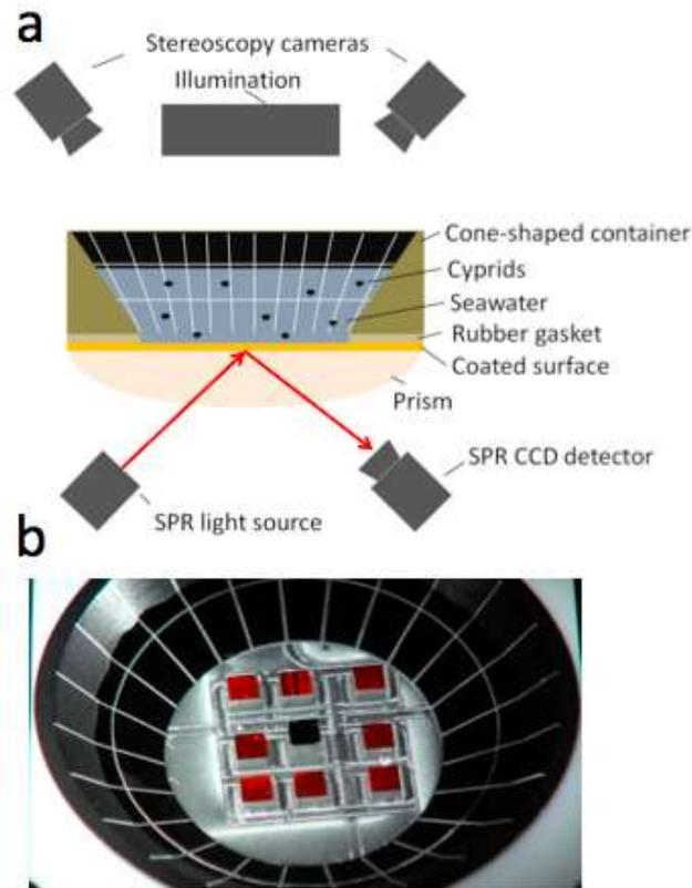
Figure 1: a) Schematic drawing of the setup. b) The cone-shaped container with coordinate grid, here shown with a calibration object at the bottom of the container. The container was designed to allow maximal field of view for stereoscopy, and at the same time easy exchange of the calibration object.
