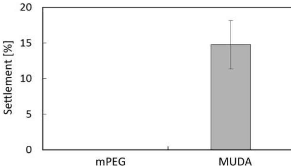
Figure 2: Cyprid settlement data after 24 h for the two surface chemistries used in the iSPR studies. Error bars represent 2 x standard error.
