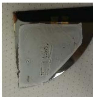
Fig 3: Delaminated porous PVDF made by phase inversion method.
