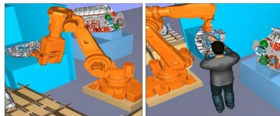
Fig. 2: Illustration of a conceptual model of a collaborative assembly cell. The operator is responsible for guiding the robot to the correct location. The robot is used as a flexible lifting device [4].
