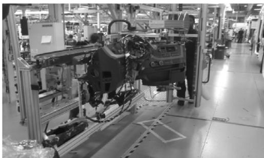
Fig. 3. The cockpit to be automatically lifted from conveyor belt, to sealing station and then inserted into the cab
