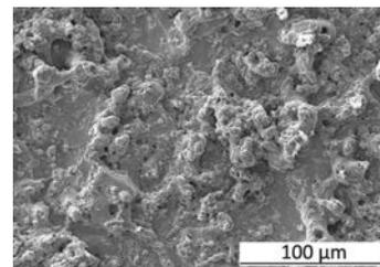
Fig. 2. Surface morphology of the EDM specimen.
