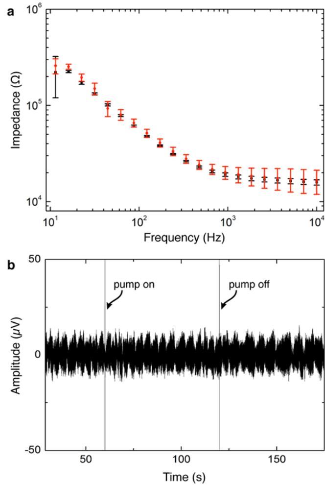
Figure 3. **Characterization of sensing electrodes incorporated into neural pixels.** (a) Bode plot of impedance versus frequency. The impedance magnitude is an average of seven electrodes. Black squares and red dots are the averaged impedance values while the OEIP is off and the while  $K^+$  is delivered ( $1 \mu A$  delivery current), respectively. (b) Time trace at a single recording site during GABA delivery ( $60 < t < 120$  s) through the sensing electrode to the ACSF target solution.
