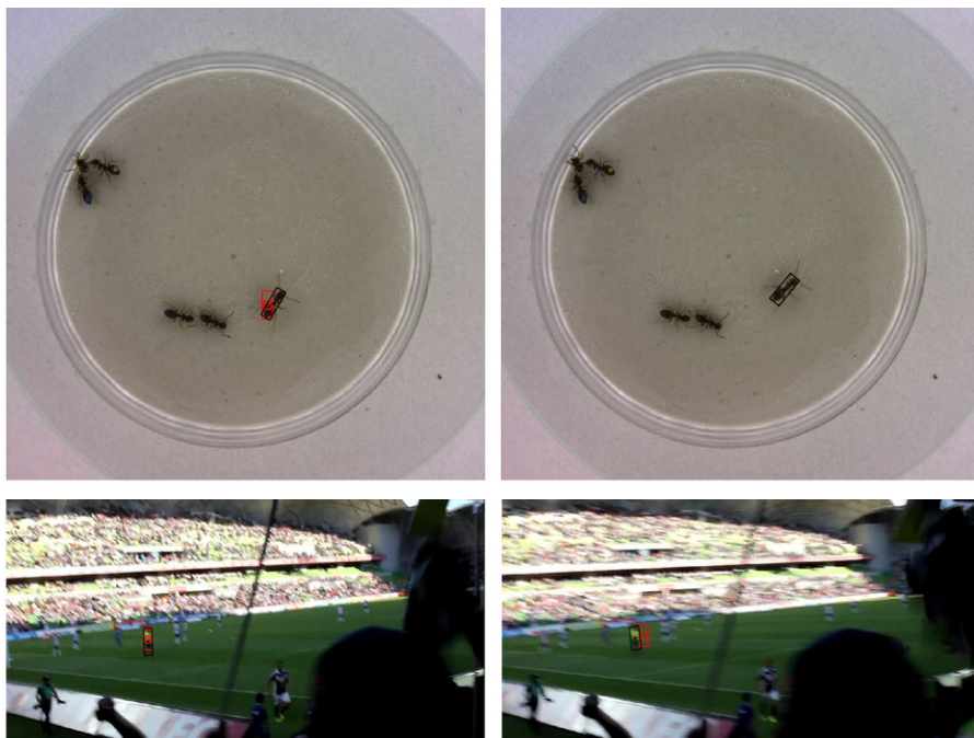
Figure 3.3: A few frames from the ants1 and the soccer2 sequences in the VOT 2017 dataset. Black bounding box is the ground-truth, red is from the DSST tracker. In the ants figure tracking fails due to the in-plane-rotation, while in the soccer case the sudden movement of the camera results in low accuracy.
