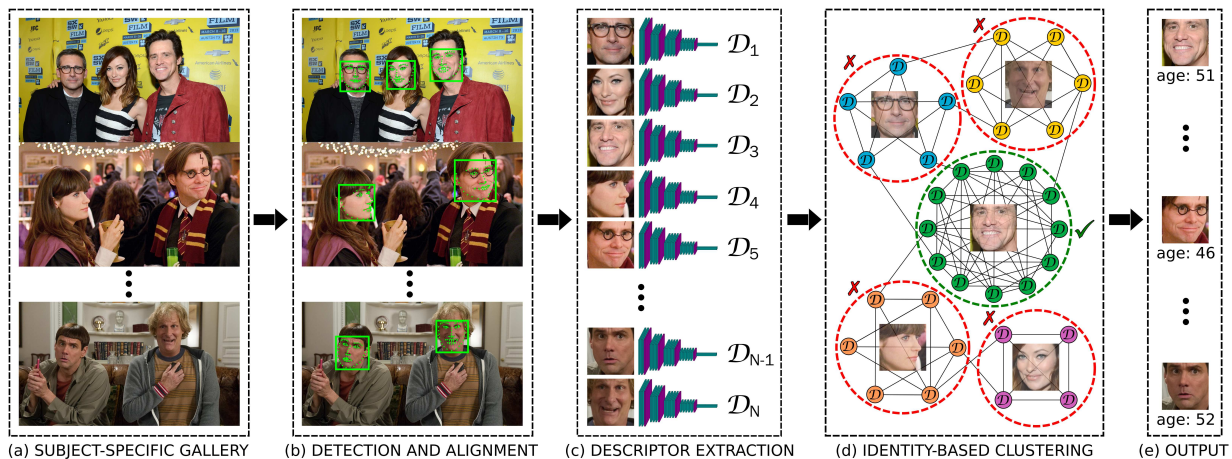
Fig. 1 The proposed unsupervised biometric filtering pipeline for the IMDB subject Jim Carrey. (a) Samples are grouped into subject-specific galleries based on the provided identity meta-data. Every image in the subject-specific gallery contains gallery’s owner (e.g. Jim Carrey), but many also contain other subjects that can be mismatched with the gallery owner’s biometric labels (e.g. age and gender). (b) Face detection and alignment of faces in the image gallery. Most of the detected faces belong to the gallery’s owner, while others are sources of label noise. (c) CNN-based face recognition descriptor extraction from all detected faces. (d) Graph-based clustering of the extracted facial descriptors. Clusters are formed based on identity matching. The gallery owner’s cluster is the largest because its face is most frequently appearing in the image gallery. (e) Samples from the largest cluster are retained, while samples from all other clusters are discarded as noise.
