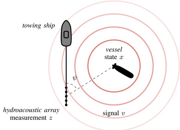
Fig. 1: The scenario considered in this paper. A hydroacoustic array is towed aft of a ship and measures the acoustic signals originating from an underwater vessel. The measurements are used in a TkBD framework to simultaneously track and detect the vessel.
