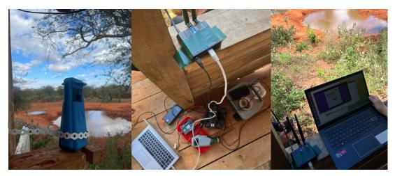
Figure 4.3: Close up at the camera, camera system connected to the router and SSH into LattePanda.
