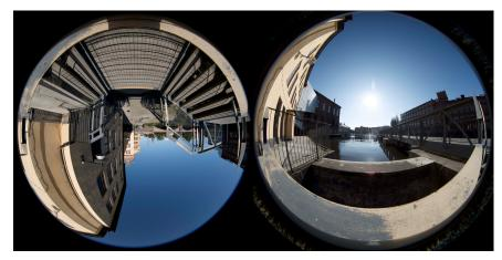
Figure 2.5: Dual fisheye image. The front camera is seen to right and the back camera to the left.
