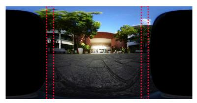
Figure 2.8: Equirectangular projection with markings for the overlap regions between the lenses. The centered image represents the front lense, while the dark parts at each side represents the back lense
