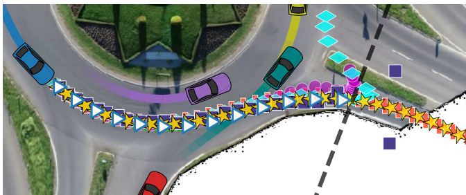
(c) Incorporating differential constraints into prediction models enhances their extrapolation capabilities. By extending the prediction horizon to t_f = 7 s, the models must compute trajectories beyond the observed data (shown by the dashed line). Although this presents a challenge for the majority of models, Trajectron++ and MTP-GO still perform well, which can be ascribed to the differential constraints within these models.
