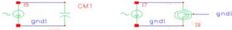
Figure 31. Schematic used for optimization of the capacitors and the inductors. A current source connected to respective passive component.
