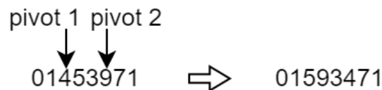
Figure 2.13: Scramble Mutation with a selected segment of length 4.
