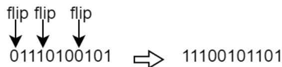
Figure 2.9: Bit-flip Mutation with 3 successful weighted coin flips.
