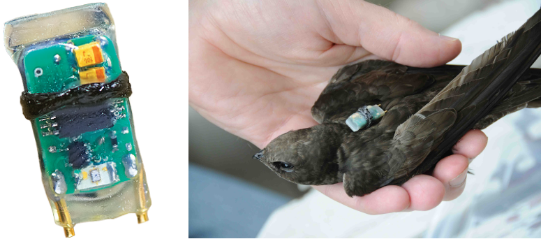
Figure 1.3: A light logger consisting of a battery, memory clock and a light sensor with a weight of less than one gram, suited for bird localization 2 .
