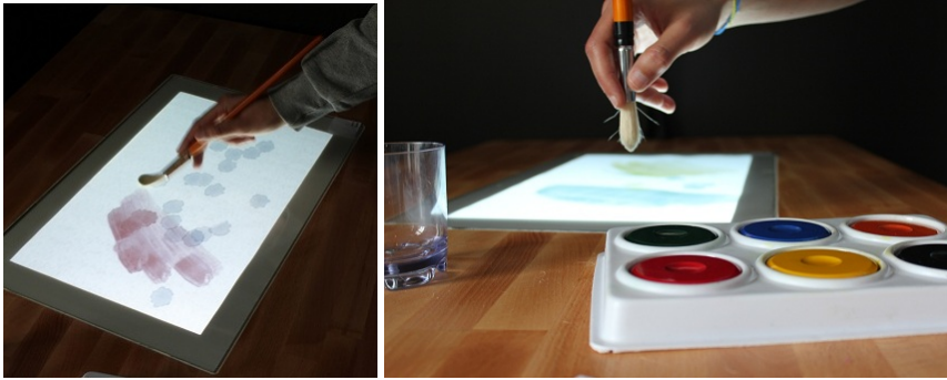
Figure 1.7: Virtual watercolor painting application where the painting is displayed on a screen. The user interacts using a regular painting brush equipped with a permanent magnet. A sensor network of four magnetometers is mounted under the screen sensing the position and orientation of the brush. The user can paint and splash color on the virtual canvas and select new colors from the palette and wet the brush in the (virtual) water glass.
